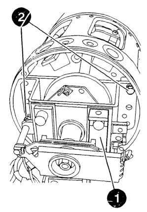
ASSEMBLING STARTING-MOTOR SOLENOID WITH CONTROL RELAY
